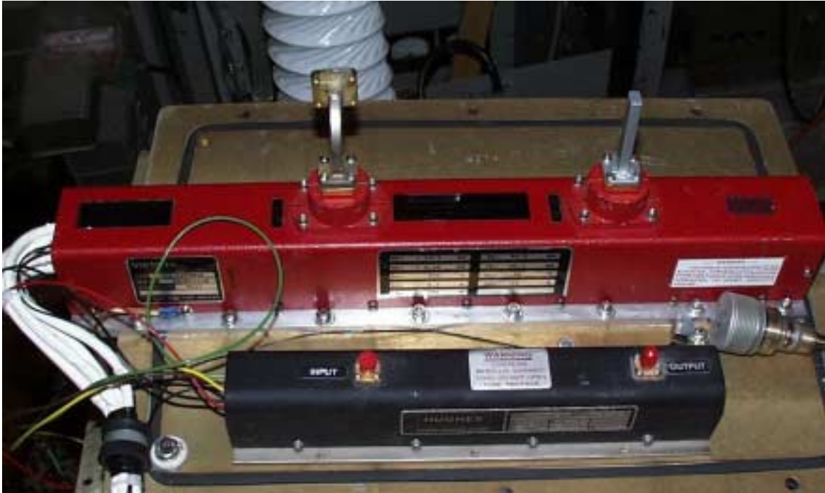
Figure 9 80 Watt 32-38 GHz Varian TWT, Hughes 10 Watt TWT & Glass 2C39 Tube
