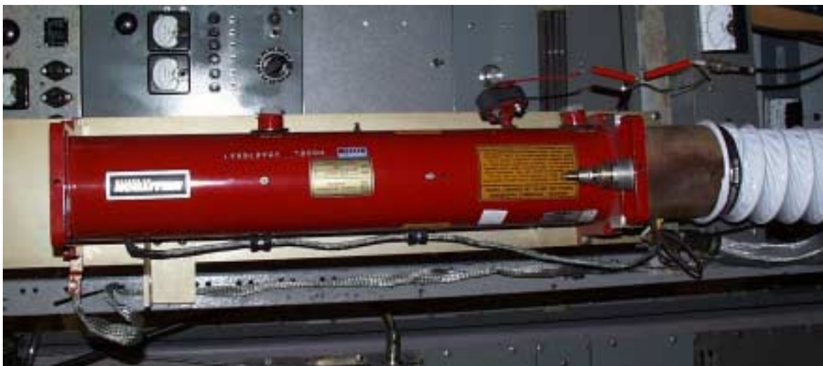
Figure 8 Varian 100 Watt 28 GHz TWT
